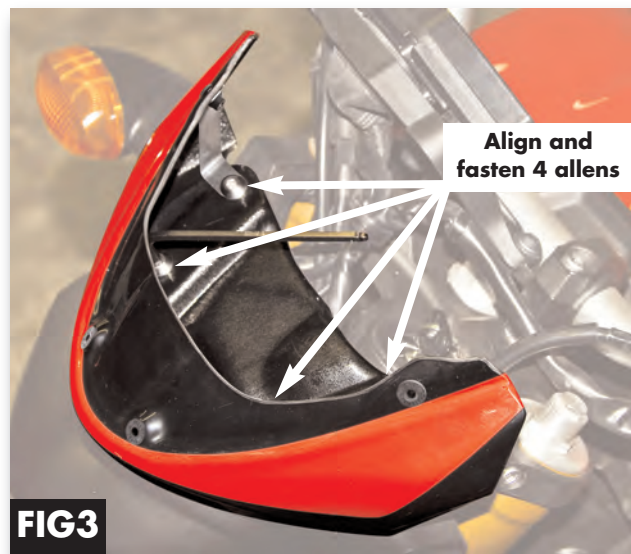
Fig 3. Place and align the ZG fairing on top of the 4 allen fastener holes, insert the four allen fasteners and tighten.
