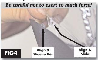
**Fig 4.** To finish the installation process, align and slide the U-hooks located upper fairing corners, into their respective slot by applying light pressure.
