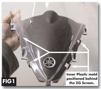
**Fig 1.** Remove both mirrors. Locate both fasteners in the inside fairing. Once you remove the mirrors the factory screen can be removed by sliding back and pulled up slightly. **For 2012 & up install:** OEM windscreens have an inner plastic mold attached to the screen (as shown above). Carefully remove it and attach to Zero Gravity screen as shown in **Fig 1.**
