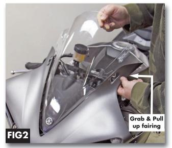
**Fig 2.** Start by inserting the windscreen from one side. To slide in, grab and pull up on the upper fairing as shown above. Rotate the mirror rubber gasket to align the side windscreen humps. Repeat for the other side. **For 2012 & up install Tip:** The trick to keeping the two plastic units together, is to not flex the windscreen during the process.
