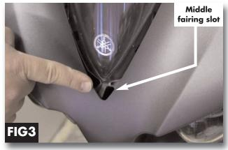
**Fig 3.** Locate the middle fairing slot at the bottom of the windscreen. Insert windscreen into this slot for positive retention.
