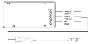
The Autotune kit when used in conjunction with the PCV allows the bike to be automatically tuned to a target air/fuel ratio. To use this feature you must first enable Auto Tune in the PCV.
