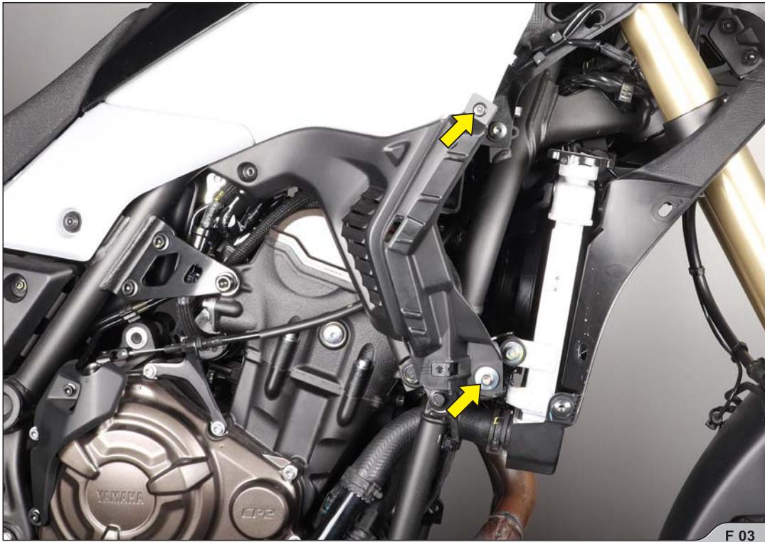
4. For euro 5 model only: undo marked plastic fastener than disconnect the lambda sensor's connector (F 04).
