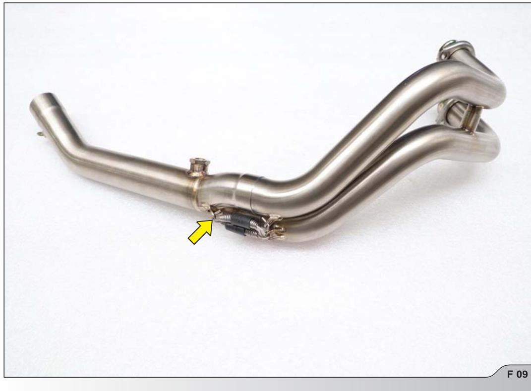
2. Install and hand tighten the headers onto the cylinder head, using stock nuts (F 10).
