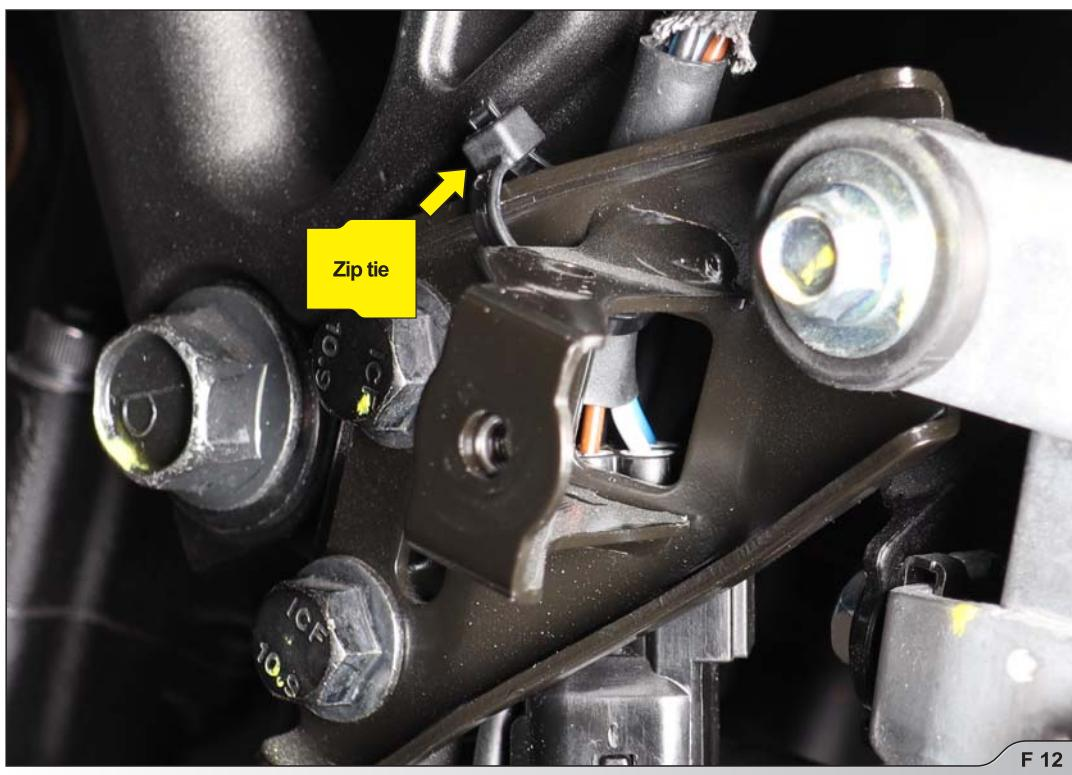
4. For euro 5 model only: connect the lambdas sensor's connector with Akrapovič extension cord. Lambda sensors electric lead should be secured only with marked plastic fasteners (**F 13**).
