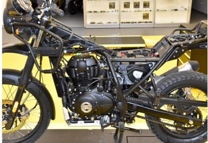
Locate the fuel injector connector under the fuel tank.
