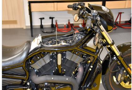
Plug the QSHconnectors in-line with the fuel injector connectors.
